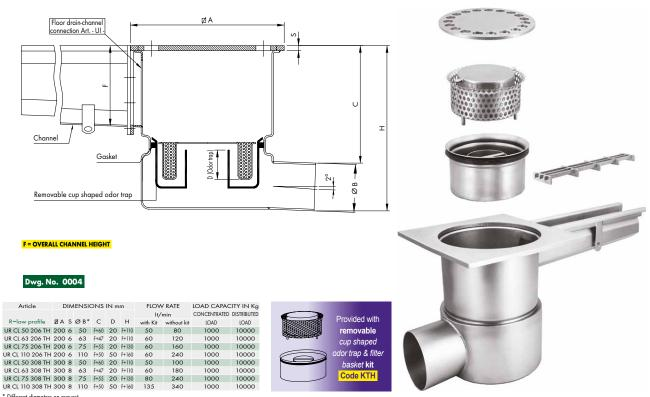
\* Different diameters on request. N.B. water seal depth (dimension D) of 50 mm in compliance with standard UNI EN 1253-1
