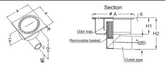
Inoxsystem® IDrain 0010 - Floor drain with 6 mm thick perforated solid cover - square shape - visible edges - horizontal outlet with odor trap - removable filter Н1 H2 Flow rate Removable Width Ø Outlet Length Length lt/min cover ID40L106 100 40 85 40 12 Perforated plate ID50L156 45 50 150 100 40 Perforated plate Dwg, No. 0010 - Made of: Aisi 304 stainless steel, 2 mm thick - Aisi 316 on request
