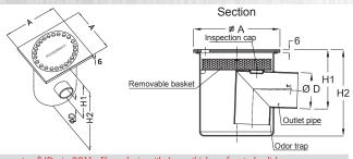
Inoxsystem® IDrain 0011 - Floor drain with 6 mm thick perforated solid cover - sq shape - visible edges - ultra-lowered horizontal outlet with odor trap - removable filter Н1 H2 D Flow rate Removable Width Ø Outlet Length Length lt/min IDL4025106 90 12 Perforated plate IDL5025156 150 75 110 50 40 Perforated plate
