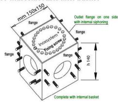
\* Upon request: can be used all floor drains described on page 10 in this case indicate the quantity and location of flanges necessary (90°-180°-270°-360°)
